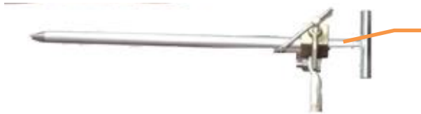
Spike with a grounding device
